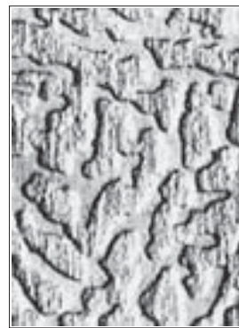
Surface. Centre. Uddeholm Impax Supreme Ø 500 mm (20").
