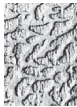
Surface. Centre. Uddeholm Impax Supreme Ø 500 mm (20").
