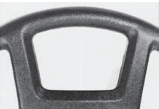
Part of an automobile steering wheel produced from a photo-etched Uddeholm Impax Supreme mould.
