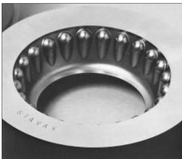
Fig. 14. This Uddeholm Stavax ESR mould insert was finished by EDM "polishing".
