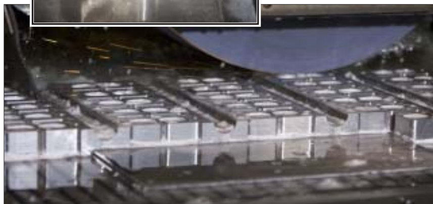
Fine grinding of details in hardened Udddeholm Mirrax ESR
