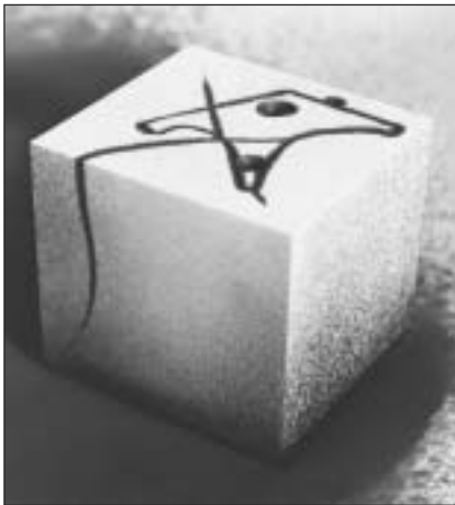
Fig. 12. This block of D2 steel, approx. 50 x 50 x 50 mm (2" x 2" x 2"), cracked during the wire EDM operation.
