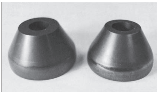
PVD coated tools in Uddeholm Vanadis 23 SuperClean for cold forming of tubes.
