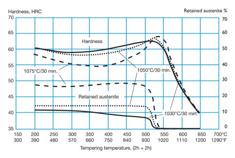
Above tempering curves are obtained after heat treatment of samples with a size of  $15 \times 15 \times 40$  mm, cooling in forced air. Lower hardness can be expected after heat treatment of tools and dies due to factors like actual tool size and heat treatment parameters.
