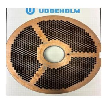
» After 102 days production Non working side on hole plate still in very good condition (coating helps against corrosion)
