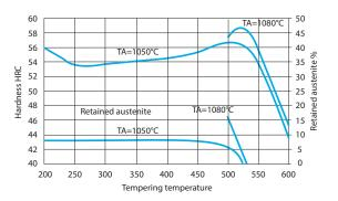
The tempering curve is obtained after heat treatment of samples with a size of  $15 \times 15 \times 40$  mm, cooling in a vacuum furnace.
