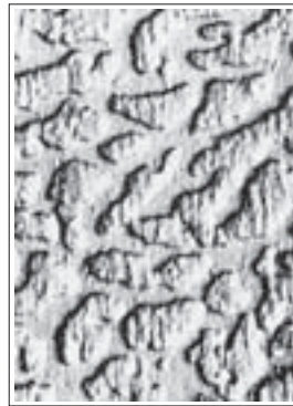
Surface. Centre. Uddeholm Impax Supreme Ø 500 mm (20").
