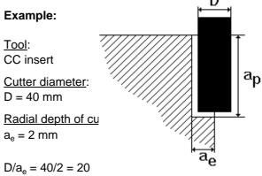
Feed acc. to table slot milling = 0.11 mm/tooth Correction factor acc. to chart:  $C_f = 2.8$
