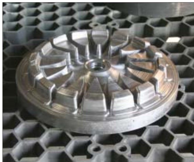
A lower die for aluminium rim just before heat treatment on charging grid. Photo: ASSAB Çelik (Turkey)
