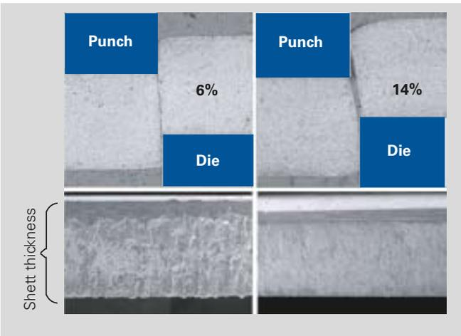
Figure 3-10. Edge cut with varying die clearance.
