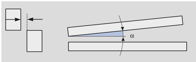
Figure 3-25. Cutting clearance and shearing angle respectively.
