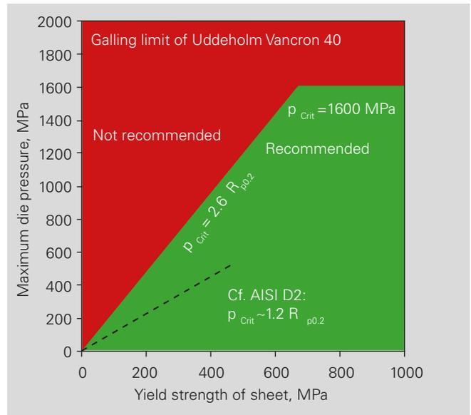
Figure 3-5b. Limits to guide the use of uncoated Uddeholm Vancron 40 to form carbon steel. Recommendations are based on application tests and FEM simulation. For comparison the approximate level of the galling limit of uncoated AISI D2 tool steel is included.
