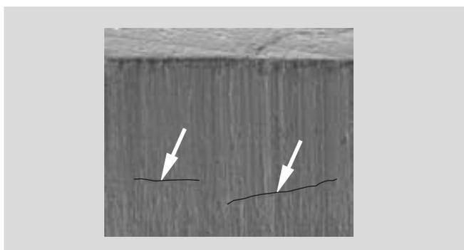
*Figure 3-14. Cracking developed as a result of fatigue.*
