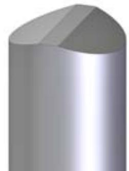
Figure 3-20. A chamfered punch with a flat centre section.
