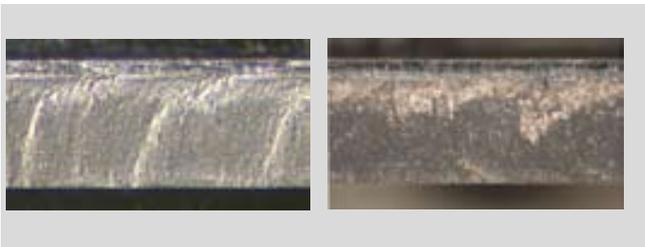
Figure 3-30. Sheet edge appearance for Docol 1400M, t=2 mm with different cutting conditions. The left image indicate that cutting clearance and/or shearing angle is too large. The right image indicate that the cutting conditions are OK.
