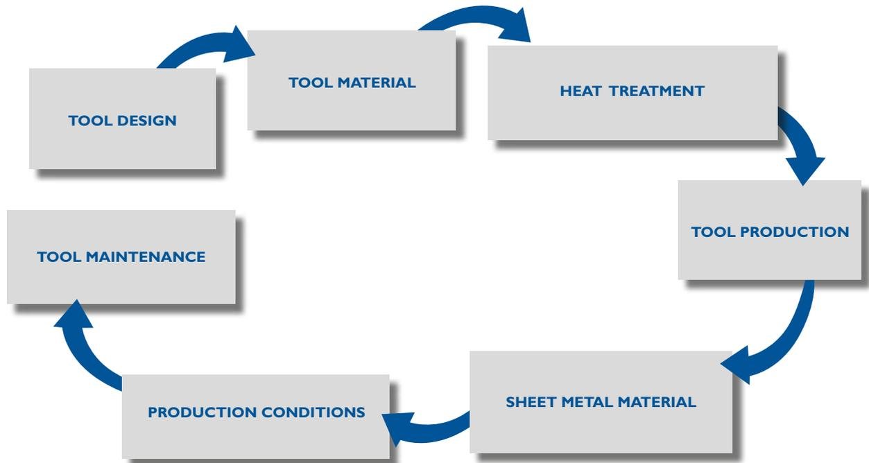
*Figure 3-1. Process steps from tool design to tool maintenance.*
