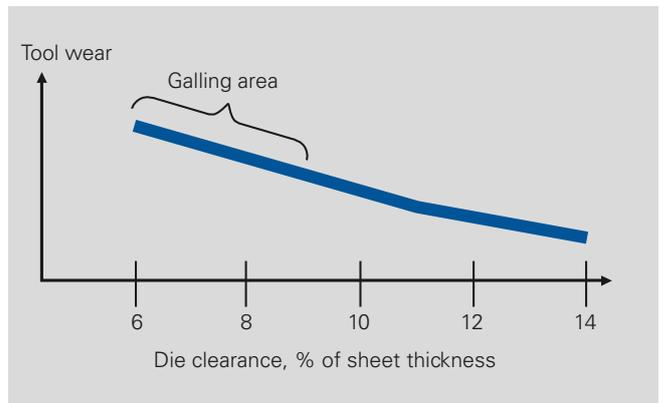
Figure 3-11. Relation between tool wear and die clearance when blanking in Docol 800 DP (sheet thickness = 1 mm).
