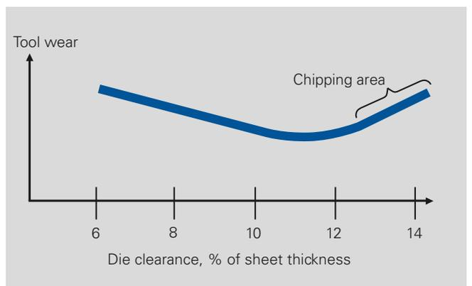
Figure 3-12. Relation between tool wear and die clearance when blanking in Docol 1400 M, with sheet thickness 1 mm.
