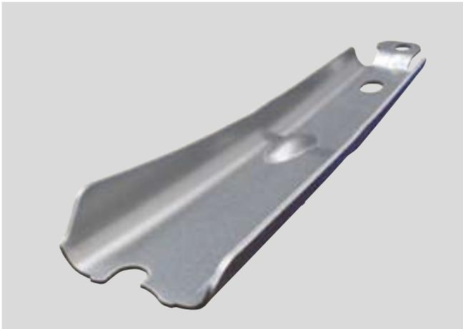
Figure 3-33. B-pillar reinforcement.
