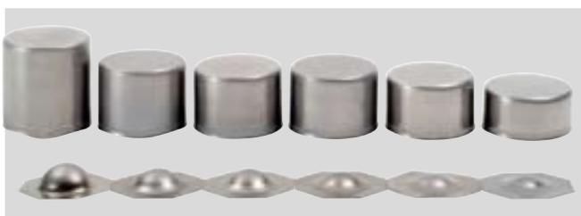
*Figure 3-3. Maximum- cup height and dome height for deep drawing and stretch forming, respectively. Steel grades (from left to right): DC06, Docol 600 DP, Docol 800 DP, Docol 1000 DP, Docol 1200 M and Docol 1400 M*
