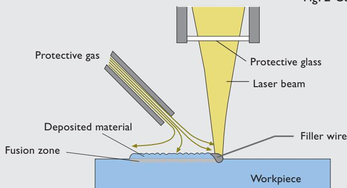
Fig. 3 Laser Welding
