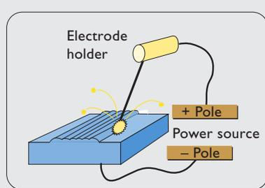
Fig. 1 Shielded Metal-Arc Welding SMAW (MMA)
