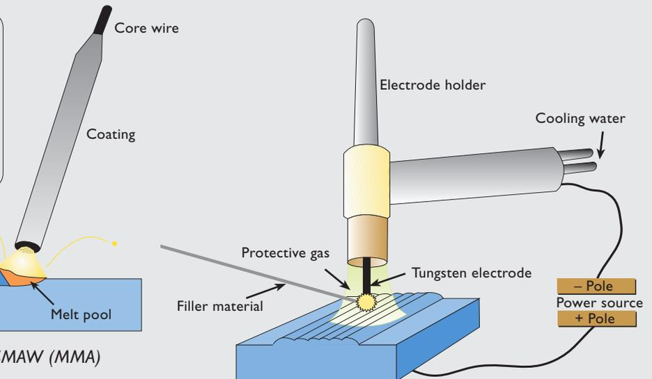
Fig. 2 Gas Tungsten Arc Welding GTAW (TIG)
