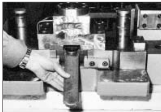
Cold cropping tool made from Uddeholm Viking.
