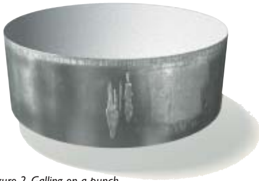
Figure 2. Galling on a punch.
