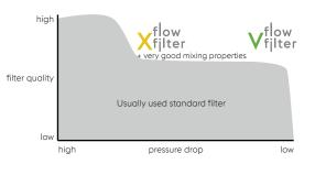
Pressure drop and shear stress can be influenced by many parameters (eg injection material, filler material, temperature, etc).
