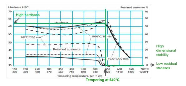
Fig. 4. Dimensional stability Uddeholm Sleipner
