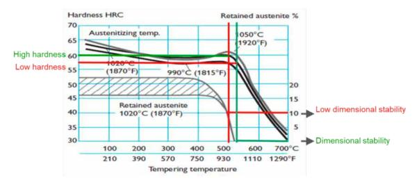
Fig. 3. Dimensional stability AISI D2
