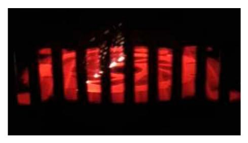
GE Additive Arcam EBM HT processing of Uddeholm Vanadis 4 Extra at 950°C
