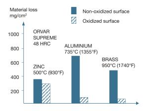
EROSION BY MOLTEN CASTING METAL Erosion is a form of hot mechanical wear on the die surface, resulting mainly from the motion of the melt.
