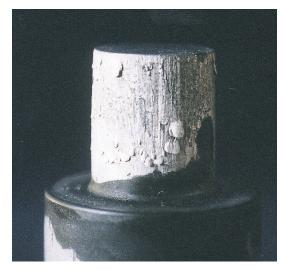
Soldering damage on a core pin.
