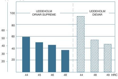
Fracture toughness at room temperature (centre, short-transverse direction).
