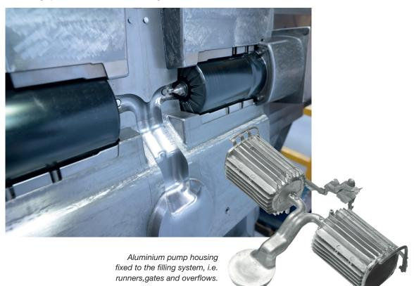
Tool for high pressure aluminium die casting.
