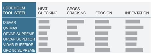
Qualitative comparison of resistance to different die failures (the longer the bar, the better).
