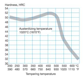
Above tempering curves are obtained after heat treatment of samples with a size of 15 x 15 x 40 mm, cooling in forced air. Lower hardness can be expected after heat treatment of tools and dies due to factors like actual tool size and heat treatment parameters.
