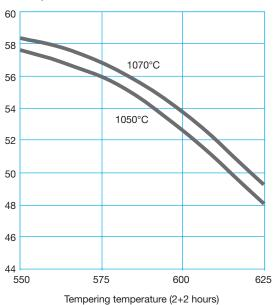
Tempering at  $250^{\circ}$ C ( $485^{\circ}$ F), 2 + 2 h gives a hardness of 56–58 HRC.
