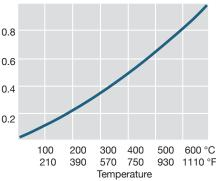
Effect of temperature on the linear expansion of Uddeholm ORVAR Supreme, soft annealed.
