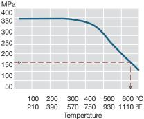
Effect of temperature on the yield strength of Uddeholm Orvar Supreme, soft annealed.
