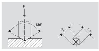
Principle of Vickers hardness testing.
