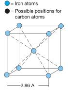
Unit cell in a ferrite crystal. Body centred cubic (BCC).
