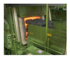
Batch type furnace with controlled atmosphere. Photo: Bodycote Stockholm, Sweden.
