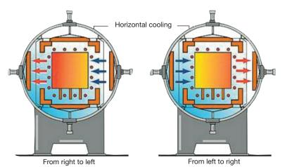
Cooling phase. Nitrogen gas stream passes through the heating chamber in different directions. Illustration from Schmetz GmbH Vacuum Furnaces, Germany.
