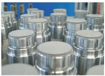
Batch prepared for heat treatment. Photo: Böhler Uddeholm Czech Republic.
