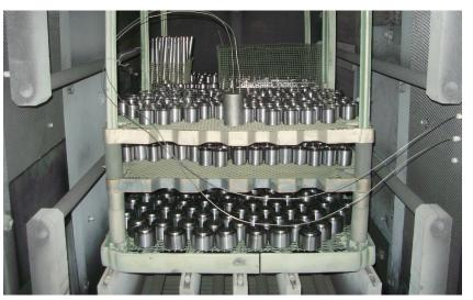
The use of thermocouples gives an overview of the temperature in different areas during heat treatment. Photo: Böhler Uddeholm Czech Republic
