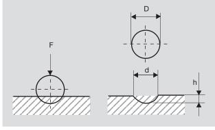
Principle of Brinell hardness testing.
