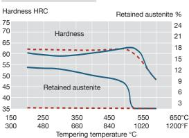
For the highest requirements on dimensional stability, sub-zero treatment in liquid nitrogen is recommended after quenching and after each tempering. Always finish with a tempering as last operation, in order to avoid the existence of untempered martensite in the part.
