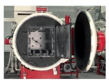
Hot zone with graphite insulation. Photo: Schmetz GmbH Vacuum Furnaces, Germany.
