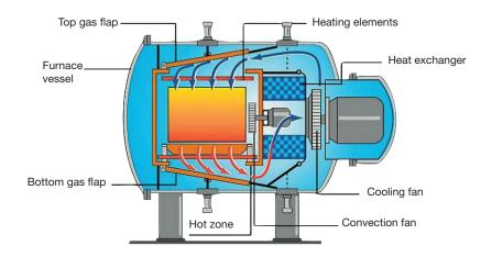
Cooling phase, top cooling. Illustration from Schmetz GmbH Vacuum Furnaces, Germany.
