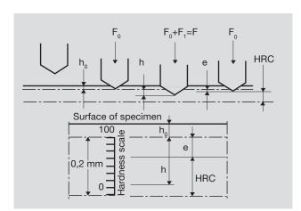
Principle of Rockwell hardness testing.
