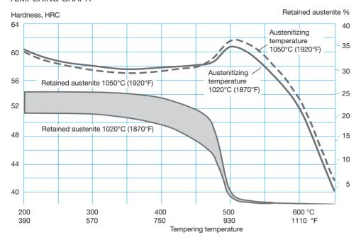
The tempering curves are obtained after heat treatment of samples with a size of 15 x 15 x 40 mm, cooling in forced air ( $T_{800-500} = 300$  sec.). Lower hardness can be expected after heat treatment of tools and dies due to factors like actual tool size and heat treatment parameters.
