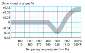
*Note*: The dimensional changes occurring during hardening and tempering are cumulative.
