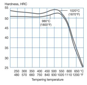
Above tempering curves are obtained after heat treatment of samples with a size of  $15 \times 15 \times 40$  mm, cooling in forced air. Lower hardness can be expected after heat treatment of tools and dies due to factors like actual tool size and heat treatment parameters.
