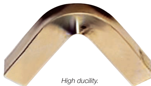
Result from un-notched charpy-v testing.
