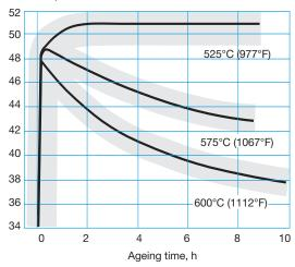
When the ageing time is reached, cool the tool in air to room temperature. Ageing at high temperature gives a better toughness compared with ageing to the same hardness at a lower temperature.
