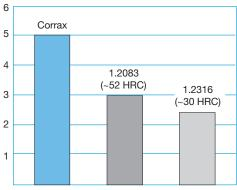
Uddeholm Corrax will withstand attacks from most corrosive plastics and diluted acids.
