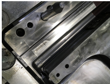
Uncoated W.-Nr. 1.2379 Clear wear marks
