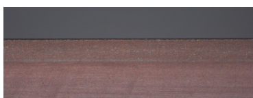
Trimming tool after 10 000 cuts Uddeholm Caldie, 61 HRC, + TiCN ultrafine Plastic deformation without Duplex coating
