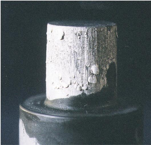
Soldering damage on a core pin.
