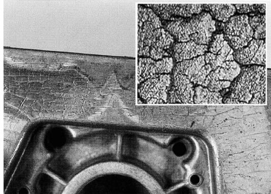
Much attention has been paid to understanding the thermal fatigue process and to relate the resistance to heat checking to basic material properties. For this purpose Uddeholm has built a special device for simulation of the thermal fatigue damage. The aim of these efforts is to improve and develop the die material and has resulted in the premium steel grades Uddeholm Dievar, Uddeholm Orvar Supreme, Uddeholm Orvar Superior, Uddeholm Vidar Superior and Uddeholm QRO 90 Supreme.
