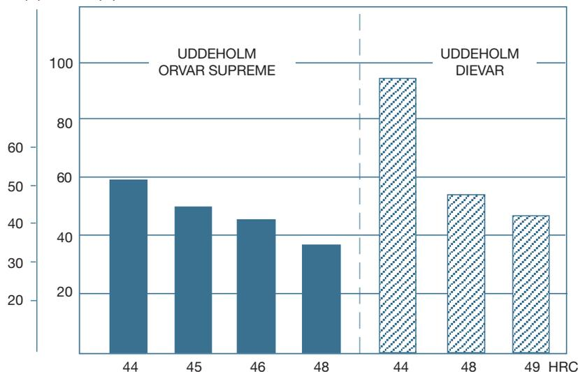
*Fracture toughness at room temperature (centre, short-transverse direction).*
