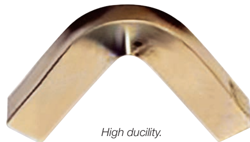
Result from un-notched charpy-v testing.
