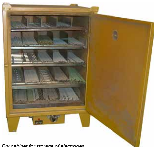
Dry cabinet for storage of electrodes.
