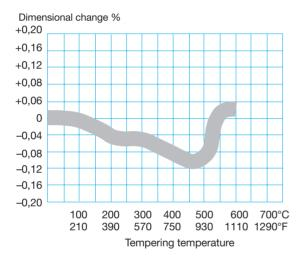
Note: The dimensional changes on hardening and tempering should be added together.
