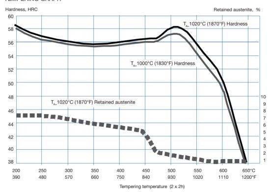
The tempering curves are obtained after heat treatment of samples with a size of 15 x 15 x 40 mm, cooling in forced air. Lower hardness can be expected after heat treatment of tools and dies due to factors like actual tool size and heat treatment parameters.
