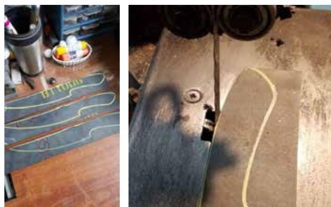
Next I epoxied some orange G10 to black peel-ply G10 for knife #1, and epoxied some grey G10 to black peel-ply G10 for knife #2. I did this so the two knives would be easier to distinguish from each other during testing. Prior to heat treating, I also had time to drill the hardware and lanyard holes in the handle material.
