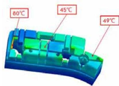
Since it is now clear that the benefits from the design possibilities of additive manufacturing technology can solve thermal problems better than high thermal conductivity materials is the low thermal conductivity of a tool steel not an issue anymore and inserts with excellent cooling efficiency can be made by this technology.
