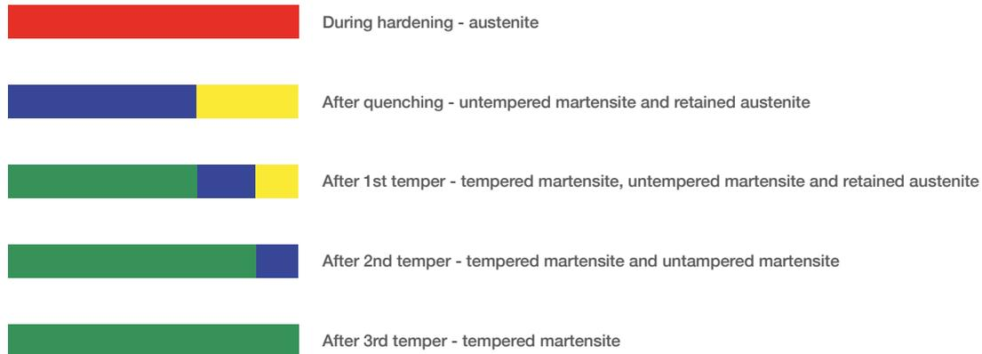
Fig. 5. Tempering of tool steel (schematic)
