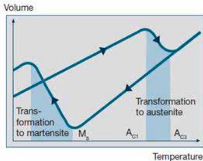
Fig. 1 Volume changes due to structural transformation
