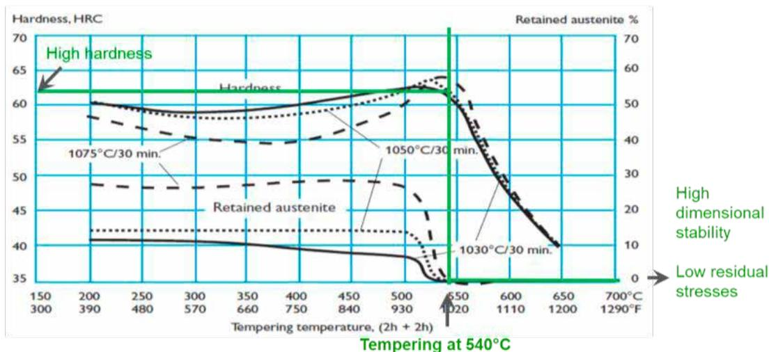
Fig. 4. Dimensional stability Uddeholm Sleiþner
