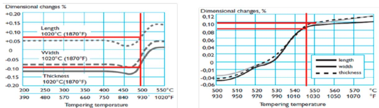
Fig. 2. Dimensional in changes conventional ingot cast steel (left), ESR and PM steels (right)
