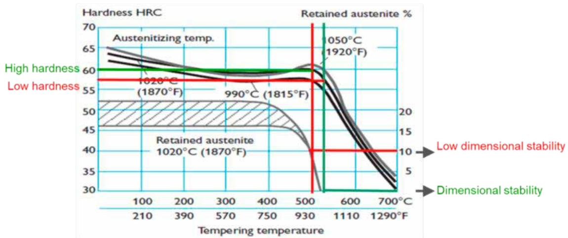
Fig. 3. Dimensional stability AISI D2
