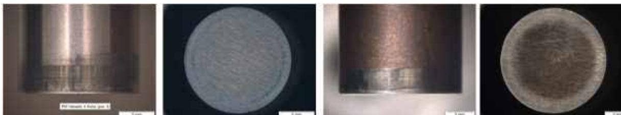
Comparison of wear of punches after 100 000 shots of CP1180 HD 1.5 mm sheet material, Uddeholm Vanadis 4 Extra PM-grade to the left and EBM processed on the right
