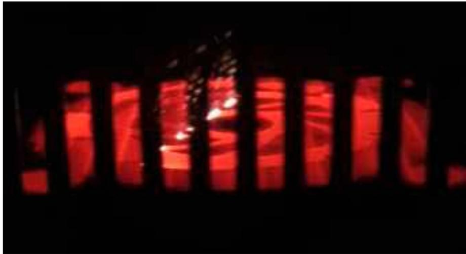
GE Additive Arcam EBM HT processing of Uddeholm Vanadis 4 Extra at 950°C
