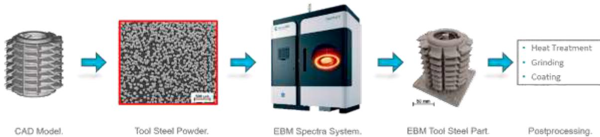
Processing route for EBM AM processing of V4E, starts with a CAD model, powder and a GE Additive EBM system
