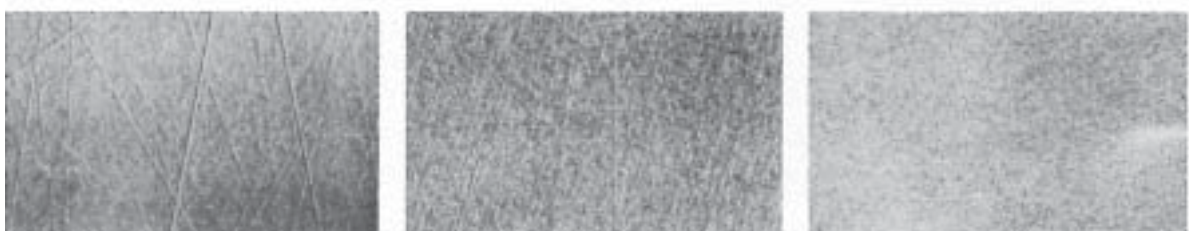
Grain size 30 \mu\text{m} Arithmetic Average micro inch 2,4
