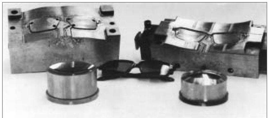
Lens mould with extreme demand on polishability. The material choice was Uddeholm Stavax ESR.
