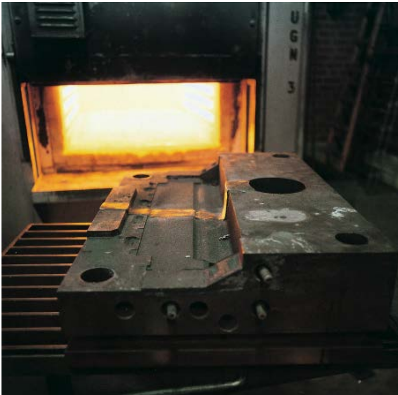
Heat treatment of a die-casting die after welding.
