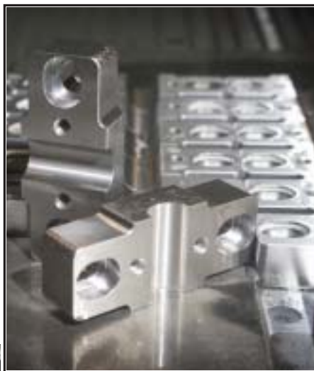
Fine grinding of details in hardened Udddeholm Mirrax ESR
