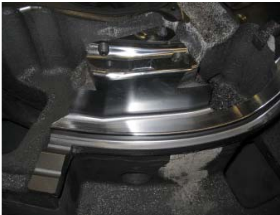
Machined Uddeholm Carmo Granshot ready for laser hardening.
