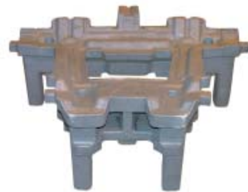
Automotive tool part cast via polystyrene model and Uddeholm Carmo Granshots, weight 750 kg.
