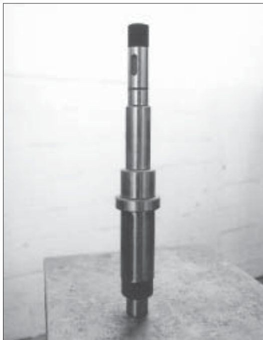
A transmission part manufactured from Uddeholm Bure, hardened to 45 HRC.
